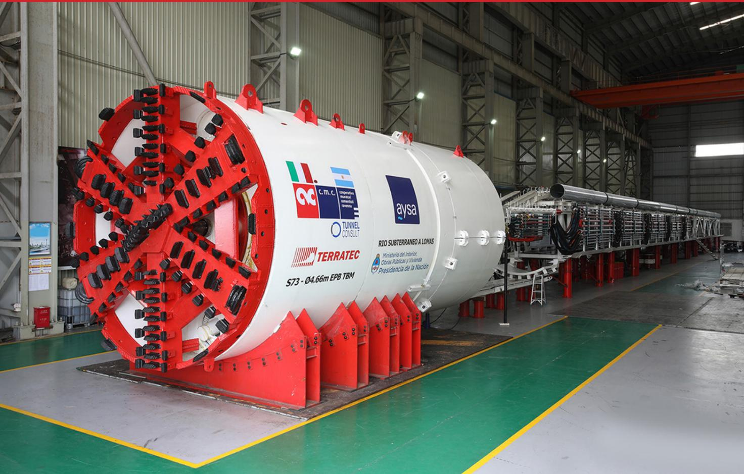
The TERRATEC EPBMs have been designed to handle the diverse soft ground geology along the project alignment, encompassing silts, sandy silts, and some cobbles. Equipped with high-torque soft ground cutterheads featuring a spoke-style design boasting a 49% opening ratio, these TBMs incorporate cutting tools comprising of multiple fixed and back-loading knife bits. This cutting-edge configuration ensures not only rapid advancement but also minimizes the need for interventions.
