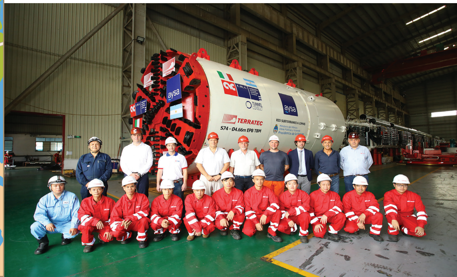
The second of two new 4.66m diameter TERRATEC Earth Pressure Balance TBMs to be delivered for a 13.5km potable water tunnel system, in Buenos Aires, Argentina.
