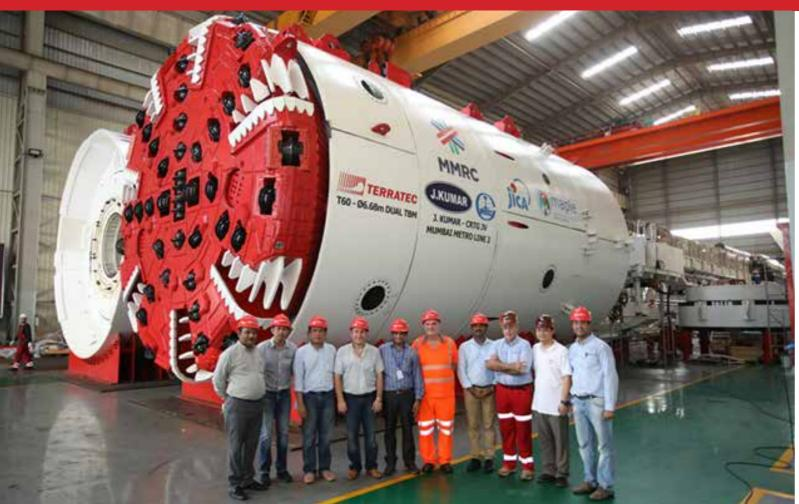
These versatile TERRATEC single shield TBMs are equipped to operate in either Open or Closed mode in the predominantly fresh and slightly to moderately weathered Basalt and Breccia that are anticipated on these contracts. The robust hard rock cutterheads are mounted with heavy duty 17" disc cutters, which are interchangeable with ripper tools, and feature large bucket openings that provide a 10% opening ratio.
