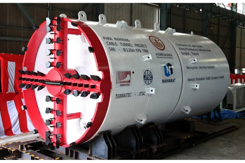
n 26th September 2016, TERRATEC celebrated the successful Factory Acceptance Test of a new 3.20m diameter Earth Pressure Balance Tunnel Boring Machine (EPBM) destined for the Phra Khanong Cable Tunnel Project in Bangkok, Thailand.
