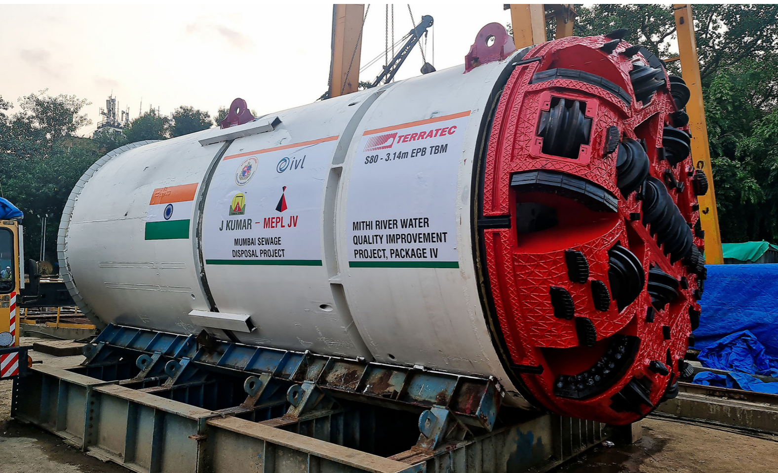
TERRATEC 3.14m diameter EPB TBM is making excellent progress for Mithi River Water Quality Improvement Project in Mumbai, India.
