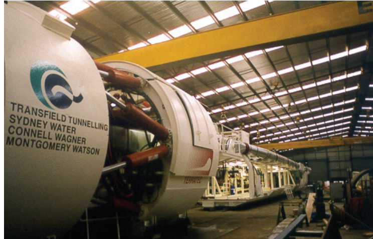
TERRATEC's Double Shield Hard Rock TBM
