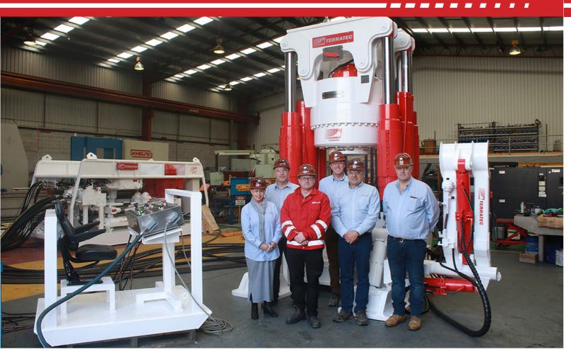
includes a powerful nearground loading pipe loader that results in a very low profile in relation to drill string length. Rotation is powered by a hollow shaft hydraulic motor, affording protection to the drill string when operating at near maximum capacity, as well as unrestricted flow of flushing water through the drive train into the drill pipe.
