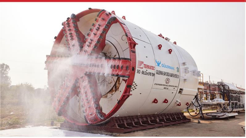
with 57% opening ratios, which had been proven to be very efficient excavating this type of soil. For added versatility, TERRATEC has designed the CutterHead to allow the cutting tools to be exchangeable for 17" disc cutters, allowing the TBM to be able to bore through the D-walls and cope with the presence of any unexpected obstacle on its way, such as old wells or foundations.
