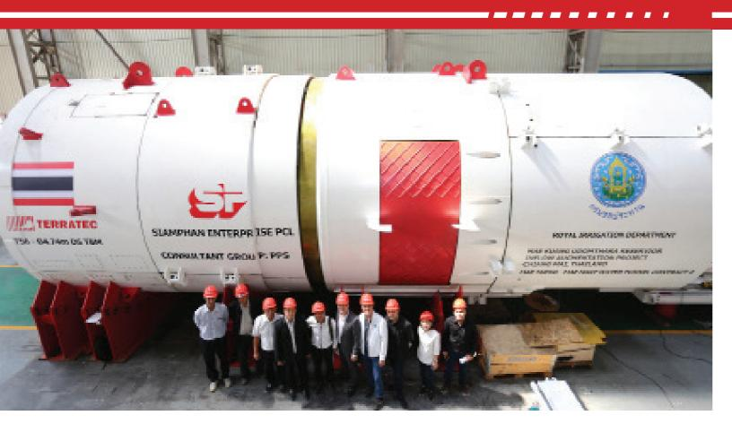
suppression. The 1,500kW Electric Variable Frequency Main Drives (VFD) will allow the Wangmontri, President of cutterheads to cut efficiently in harder rock zones at a maximum speed of 9rpm and deliver 2,896kNm of torque of to cope with fractured zones of the alignment.
