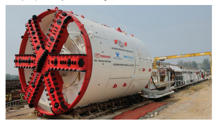
wo 6.52m diameter TERRATEC Earth Pressure Balance (EPB) TBMs are ready to be delivered to Tata-Gulermak JV, for the North-South line (Phase 1 A) of the Lucknow Metro, in India.
